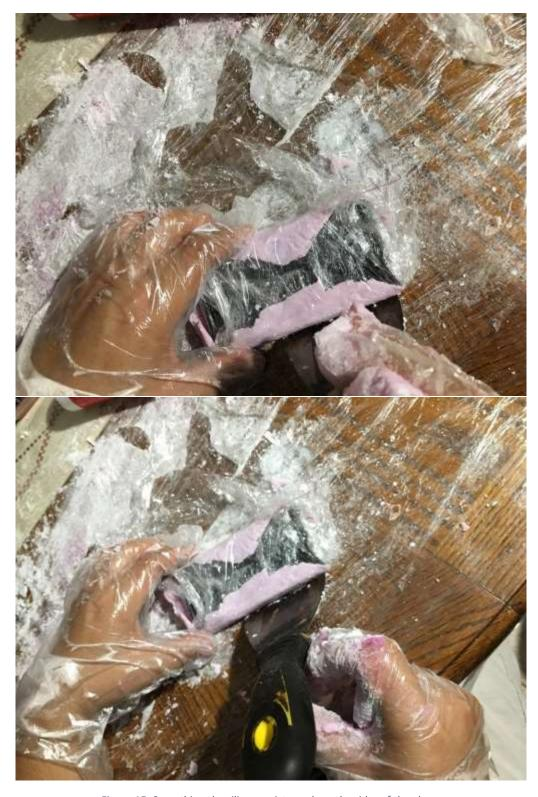
Figure 15: Smoothing the silicone mixture along the sides of the phone
