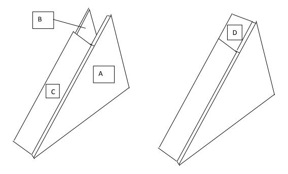
3. Glue the two stiffeners inside the ramp structure as shown in the diagram below.
