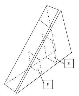
4. Glue the 7/8" strip to the ramp surface. It will take two pieces to cover the 30" length of the ramp.
