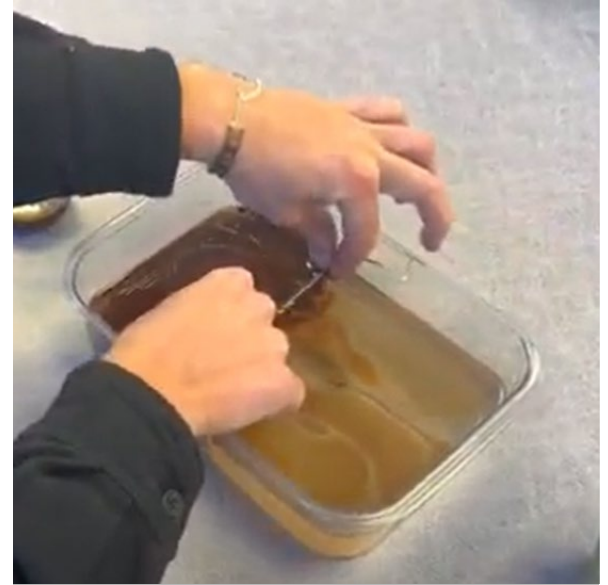
Use of a rubber band “skimmer” to separate oil and water
